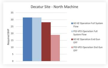
The bar graph for the Decatur Site – North Machine, shows the pump motor using 60 hertz of power both with and without a VFD when the machine is operating at full power and the end gun is on. Blue Bars – 500 GPM and 41 PSI. Red Bars – 370 GPM 61 PSI at pivot point with end gun on and 41 PSI required with end gun off. By having a VFD programmed to adjust to the decreased pressure required with the end gun off, you will save 32% of the horsepower.
