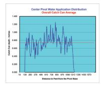
Impact Test Test Date: 5/24/18 Date Sprinklers Installed: 7/2004 Range .34" to 1.26"" Can Avg (Water Caught) .74" Uniformity 78%
